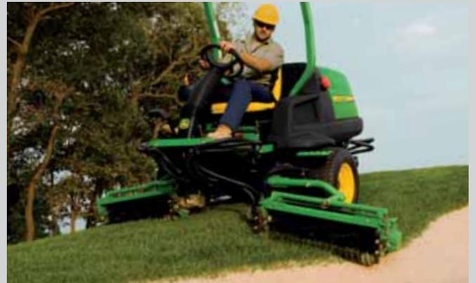
Extend individual cutting units right or left to trim around bunker edges or trees. (And skip most clean-up with walks or line trimmers.)
